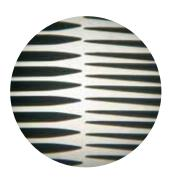
**View through the microscope** left side: pins of Top Comb Standard right side: pins of Top Comb VARIOTOP WT
